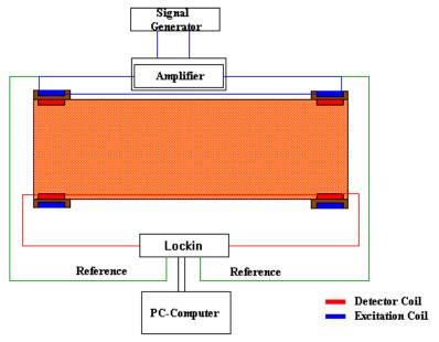
Figure 1- Alternate current biosusceptometer
